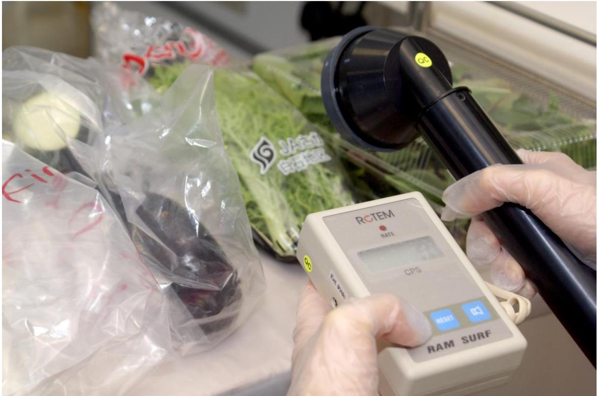
Photo 2: Testing of samples by gamma-ray spectrometer
