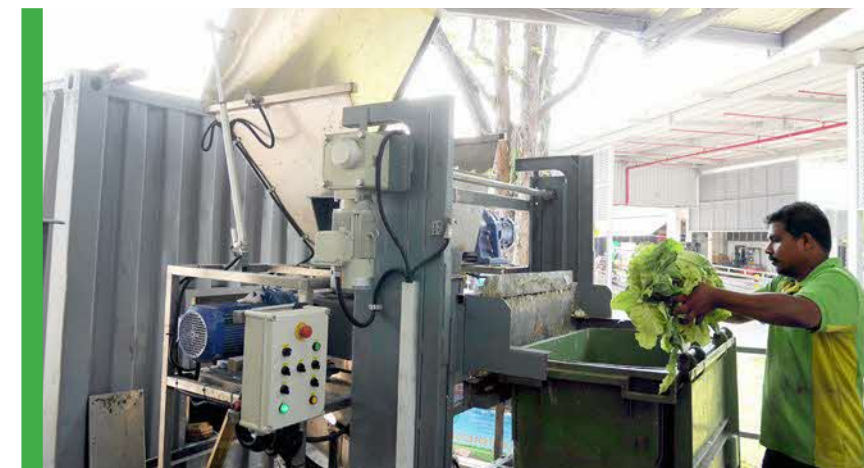
▲ Food waste is converted into compost through a food waste digester at PPWC.
